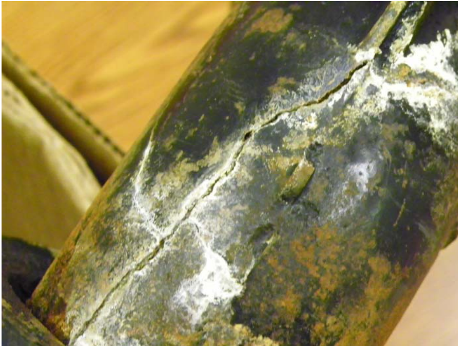
Above: A photo of one the drain pipes that was removed and replaced.
